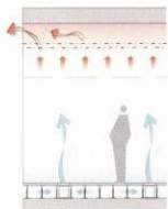
Raised floor air displacement ventilation
