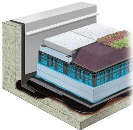
The third blue roof option is the combined green (vegetative)/ blue roof assembly where the water is jointly retained in the growing media and detained in the water storage units installed beneath the growing media and pavers. This option offers the maximum capture and management of water at the rooftop. This hides the stormwater function below the green space. The user never knows that a significant stormwater management feature is working below the green surface.
