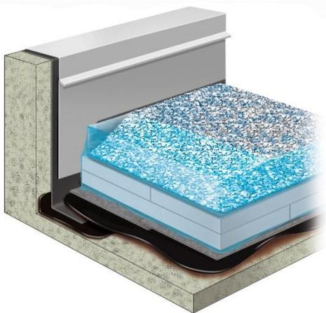
For a protected membrane roof, the water is held in the voids between the aggregates, about 30-40% of the volume according to the size of the material used. Holding water may also occur in a plaza deck assembly beneath the pavers; the water is temporarily stored in the empty space created under the pavers that are installed on pedestals.
